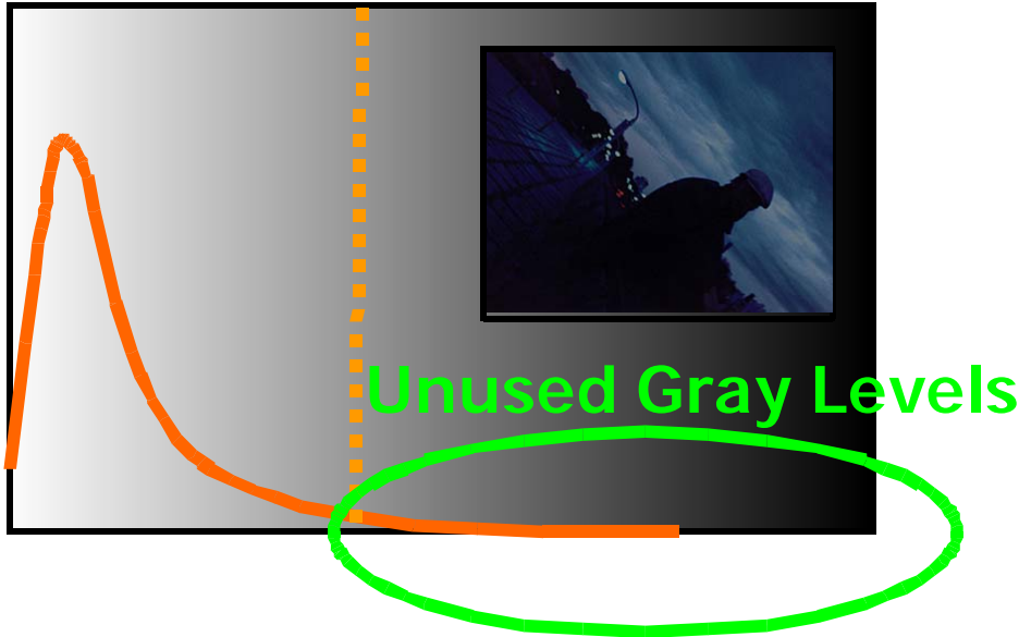
Figure 2. A dark input image before using SSBC processing technology. (Graphics from Seiko Epson Presentation.)
